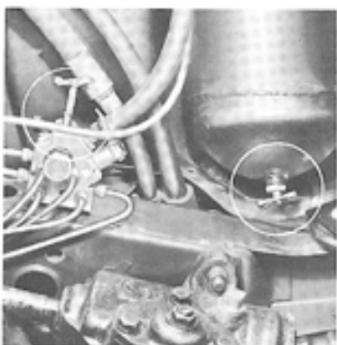
Junction Block Shut-off Valve and Accumulator Tank Shut-off Valve—(Turn clockwise to close; counter-clockwise to open)
